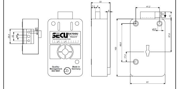
The lock is designed for use with a metal secure-storage unit and has to be mounted using screws size 6, strength category 8.8, length 35 mm. The tightening torque applied to tighten the bolts must not exceed 10 Nm. Apply a liquid screws tightening agent to stop the screws becoming loose. The lock can be mounted either horizontally, with the bolt pointing to the right or left, or vertically, with the bolt pointing up or down. The illustration above shows the lock dimensions.
