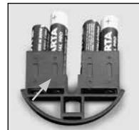
Push the cover and batteries back into the locking electronics and screw them tight.
