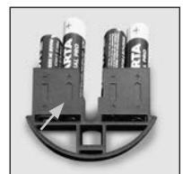
Remove the old batteries and dispose of them according to the disposal instructions on page 8. Replace the batteries with four new 1.5 V AA Mignon batteries and according to the correct polarity. For this purpose, illustrations are shown on the battery holder. Please use branded batteries and no rechargeable batteries.
