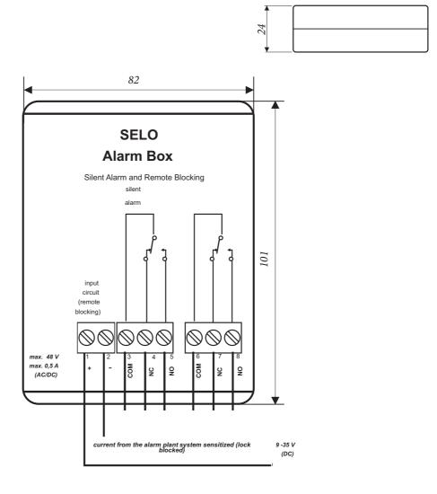
The length of the cable between the alarm box (connector) and the locking module is approximately 20 cm. Increasing the last digit of a valid user code by numerical "1" will activate the Silent Alarm of the alarm box without delay.
