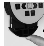
After the batteries have been changed or the housing has been opened, the change must be actively confirmed by entering the BAT code. To do this, please enter **BAT code: 228** in the input mask.
